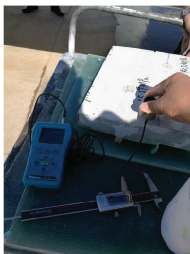
Wind Power FRP Blade Measurement (Measurement of Thickness, Curing Agent, Adhesiveness)
