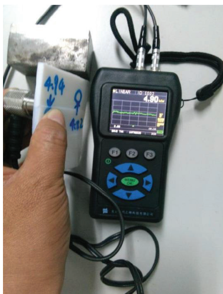
Thickness Check of PTFE
