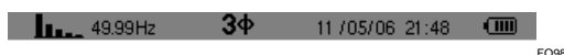
Figure 18: The 3 \phi sign at the top of the screen indicates a balanced three-phase connection configuration.
