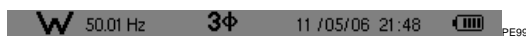
Figure 31: The 3 \phi sign at the top of the screen indicates a three-phase configuration.
