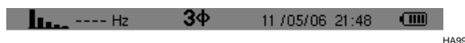
Figure 35: The 3 \phi sign at the top of the screen indicates a three-phase configuration.
