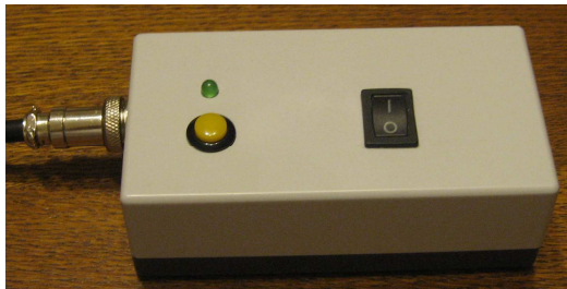
Figure 7 Battery box with ON-OFF switch and battery checker button
