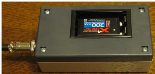
Figure 8 Bottom side of battery box for battery replacement. Always apply correct polarity when changing battery.
