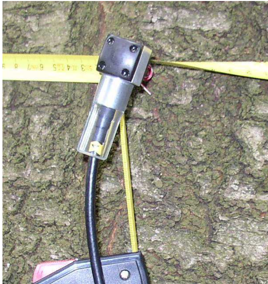
Figure 24 The way to fix the tape with the first transducer
