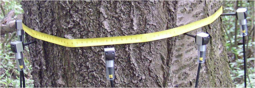
Figure 25 Sensors with tape around the trunk
