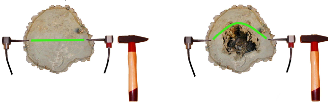
Figure 1 Sound path in healthy and decayed tree
