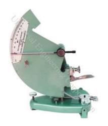
This instrument is used for measuring the resistance against tearing of **paper**, **board**, **plastic films** and other similar materials. An initial cut is made in a set of test piece, which are then torn through a given distance.
