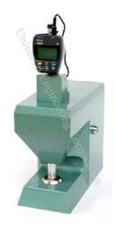
The thickness of sheet is measured as the distance between two circular plane surface, under a steady pressure 1Kg/cm² (98.0 Kpa). For rapid and accurate measurement of thickness of paper, board and plastics. Motorized, sturdy, easy to use and "push the button" operation. Digital Display, Mitutoyo (Japan) make add-on type optical transducer.
